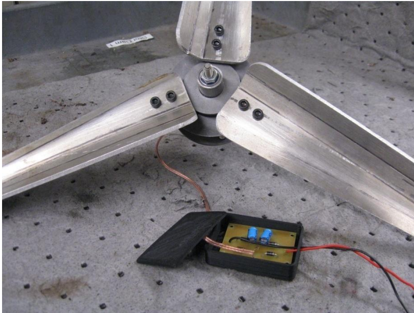
Figure 4. 3D Printed Circuit Board Potting Box
