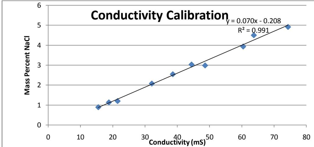
Figure 3: Conductivity meter calibration – NaCl in water
