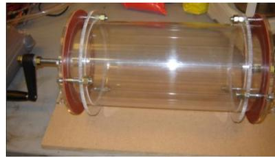
Figure 6: Tumbler apparatus for segregation demonstration
