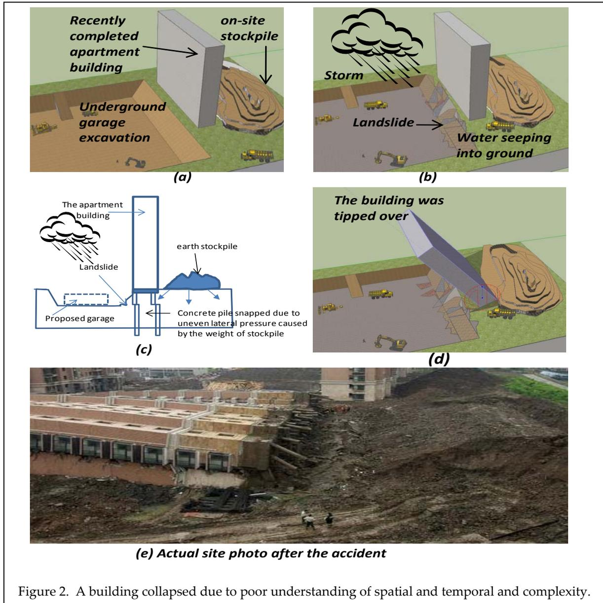
Figure 2. A building collapsed due to poor understanding of spatial and temporal and complexity.
