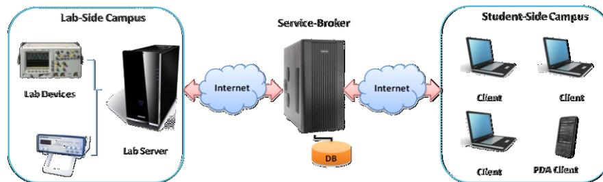
Figure 01. The iLab Shared Architecture
