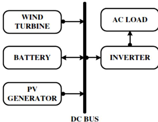
Figure 5 Project block diagram
