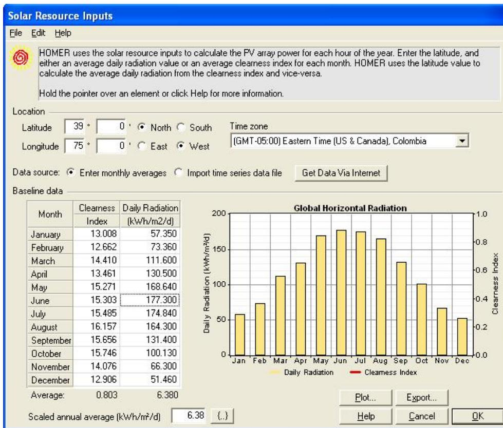
Figure 6. PV/Solar input
