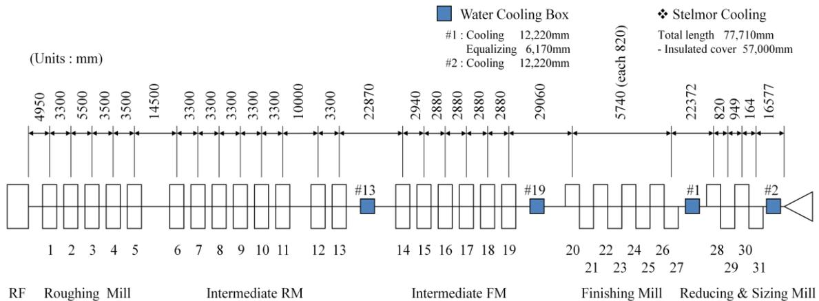
**Figure 4.** The details of the multi-stage wire rod rolling process selected for visualization in this work.
