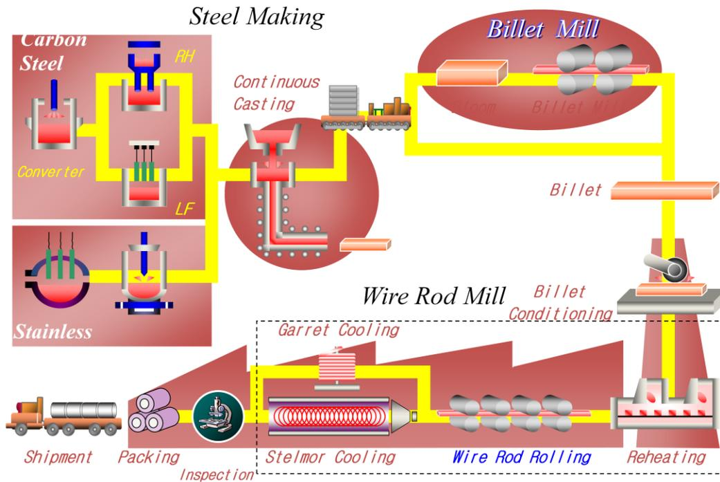
**Figure 3.** Overall process sequence to manufacture steel products. The details of the process sequence in the box above marked “**Wire Rod Rolling**” are shown in Figure 4 below.
