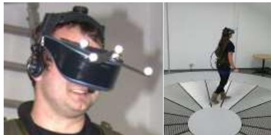
**Fig. 4.** Head Mounted Display and omnidirectional floor of the Virtual Theatre
