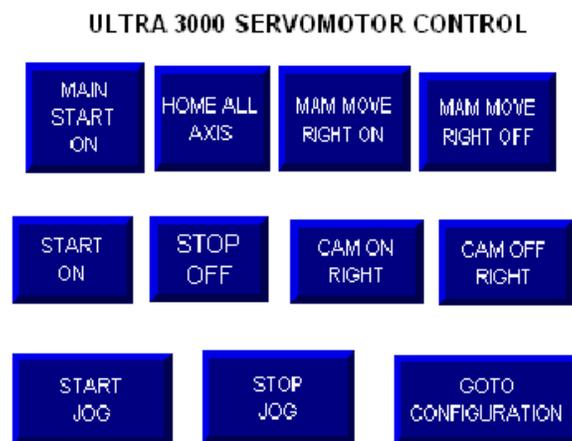
**Figure 5: A Bad HMI Touch Screen Design**
