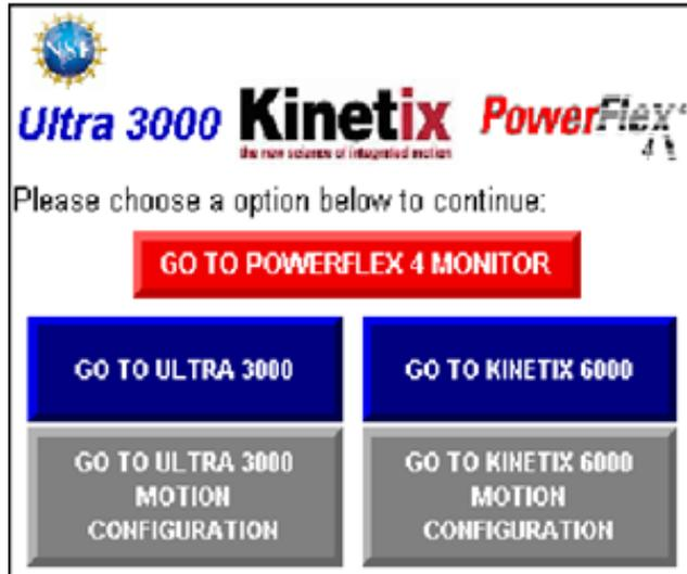
Figure 6: Allen-Bradley PanelView™ Plus 600 HMI Main Screen
