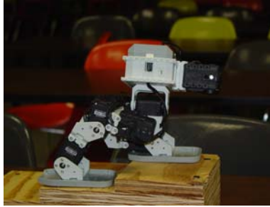
Figure 4. GERWALK robot going up stairs.
