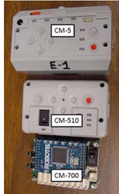
Figure 1. Current Bioloid controllers CM-5, CM-510 and CM-700.
