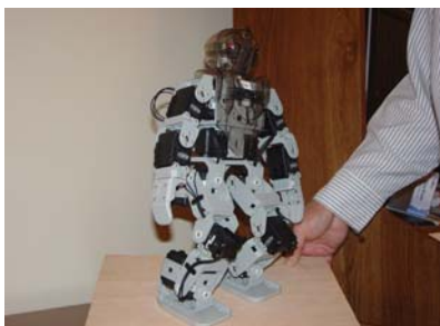
Figure 7. Humanoid robot balancing on a tilted platform using the AX-S20.
