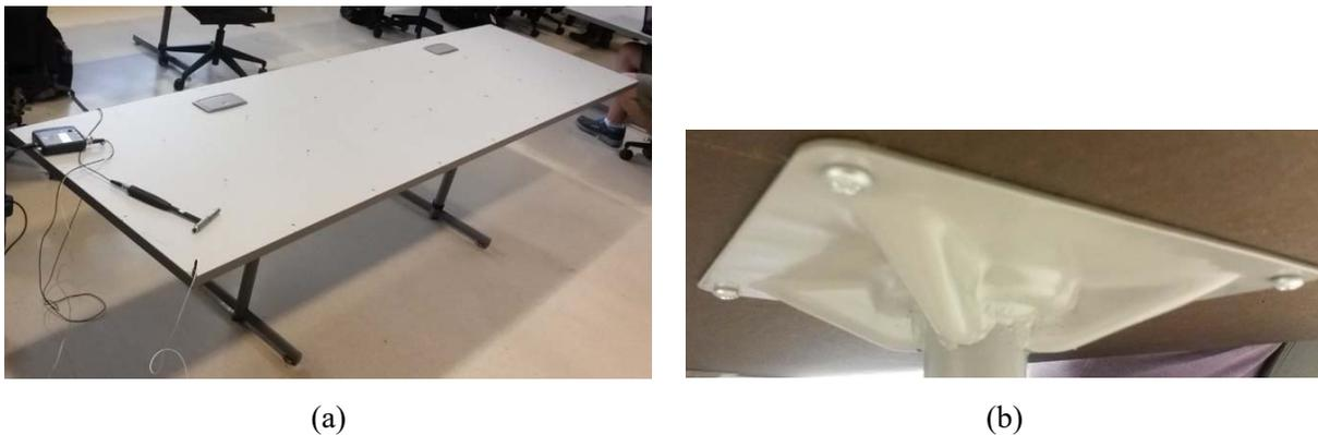
**Figure 4.** (a) A table in the lab that a team tested for their final project. (b) The legs are connected to the underside of the table by a ribbed attachment.
