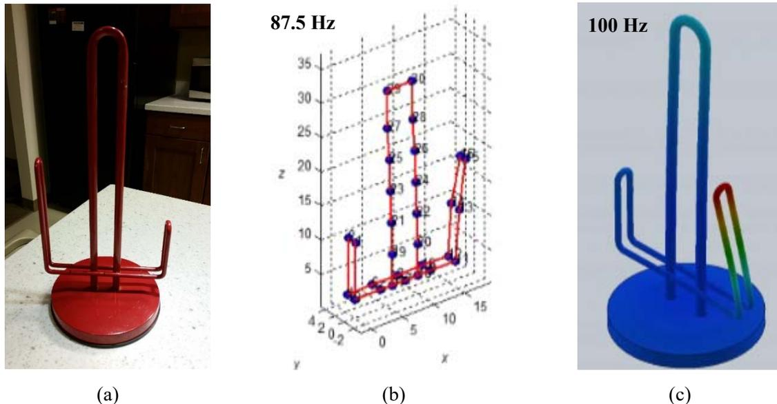
**Figure 6.** (a) A paper towel holder that a team tested for their final project. The experimental and finite element results for the first mode are shown in (b) and (c), respectively.
