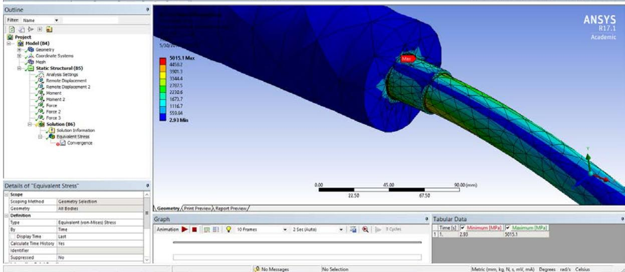
Figure 4: Problem 3-73 Bearing / Gear Flip - Constraints and Structural Analysis Results
