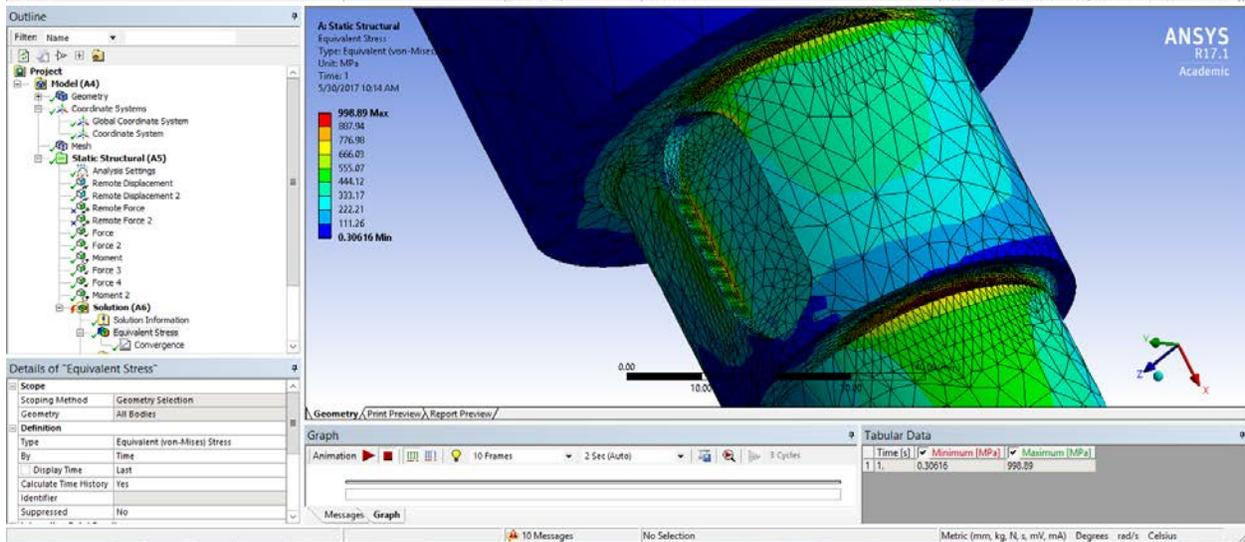
Figure 1: Problem 3-73 Shaft Max Von Mises - Constraints and Structural Analysis Results
