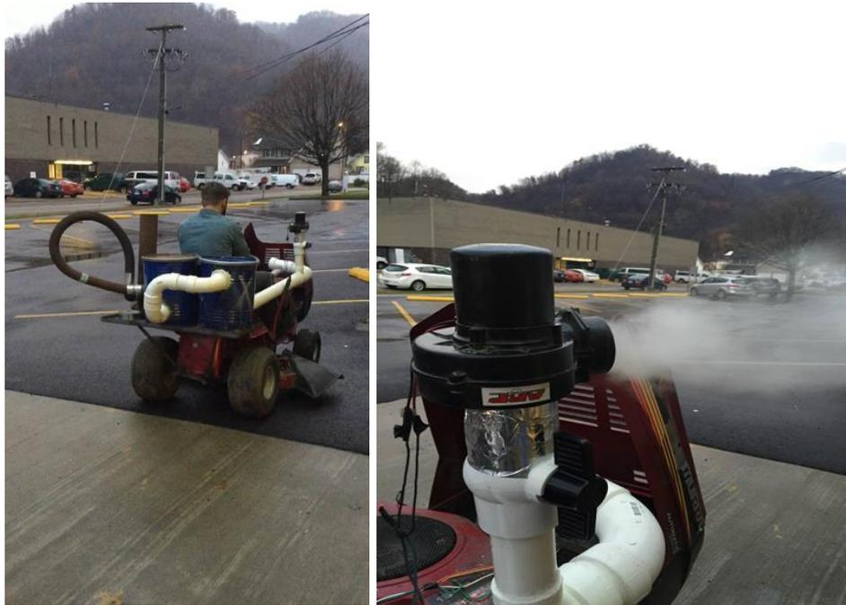
Figure 6: Biomass gasifier-based engine
