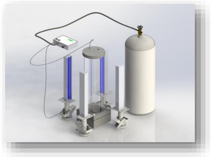
Figure 5: Schematic of the bubble column CO<sub>2</sub> capture unit utilizing microalgae
