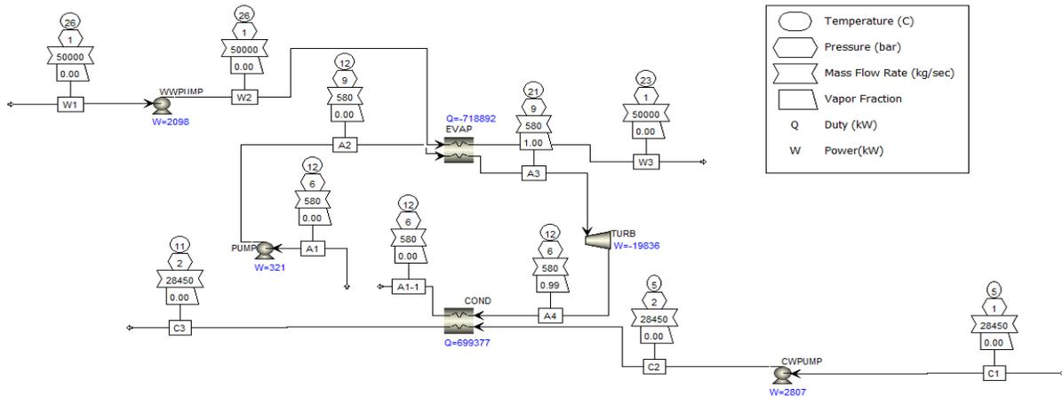
Figure 4: ASPEN Plus Model of ocean thermal energy conversion (OTEC)
