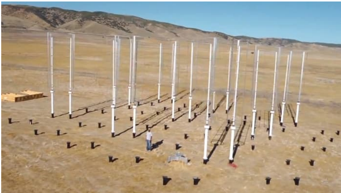
Figure 2: Caltech Field Laboratory for Optimized Wind Energy demonstrating an array of VAWTs ( http://www.gizmag.com/optimizing-wind-turbine-placement/19217/ ).
