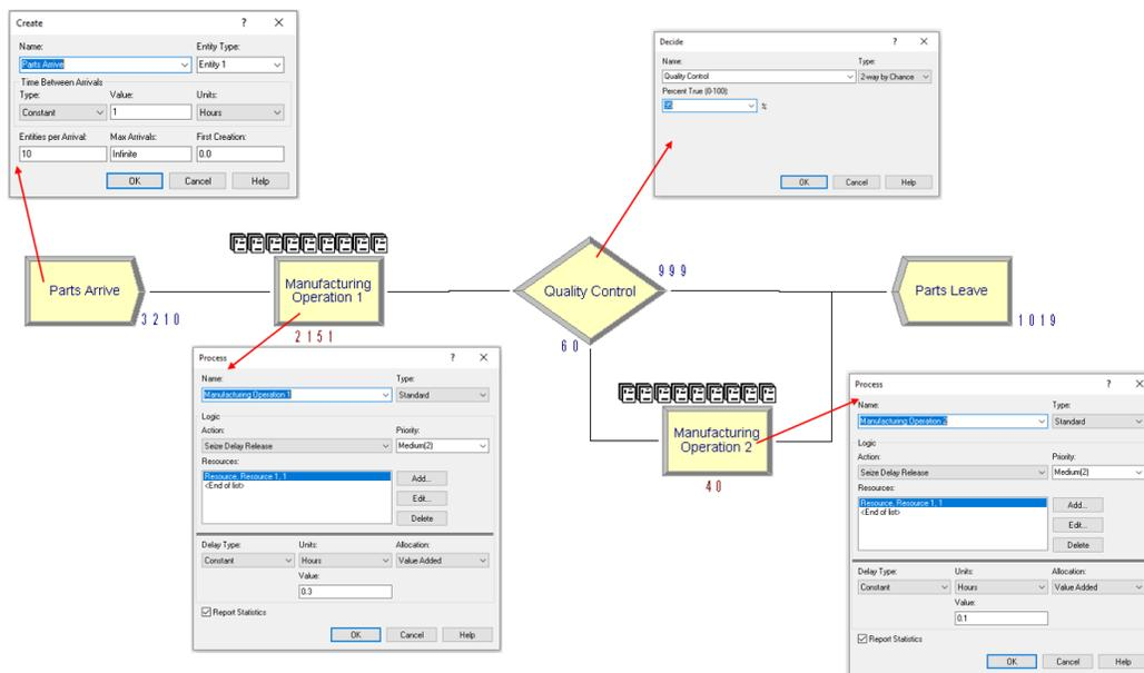
Figure 4. Manufacturing Facility with Quality Control ARENA Model
