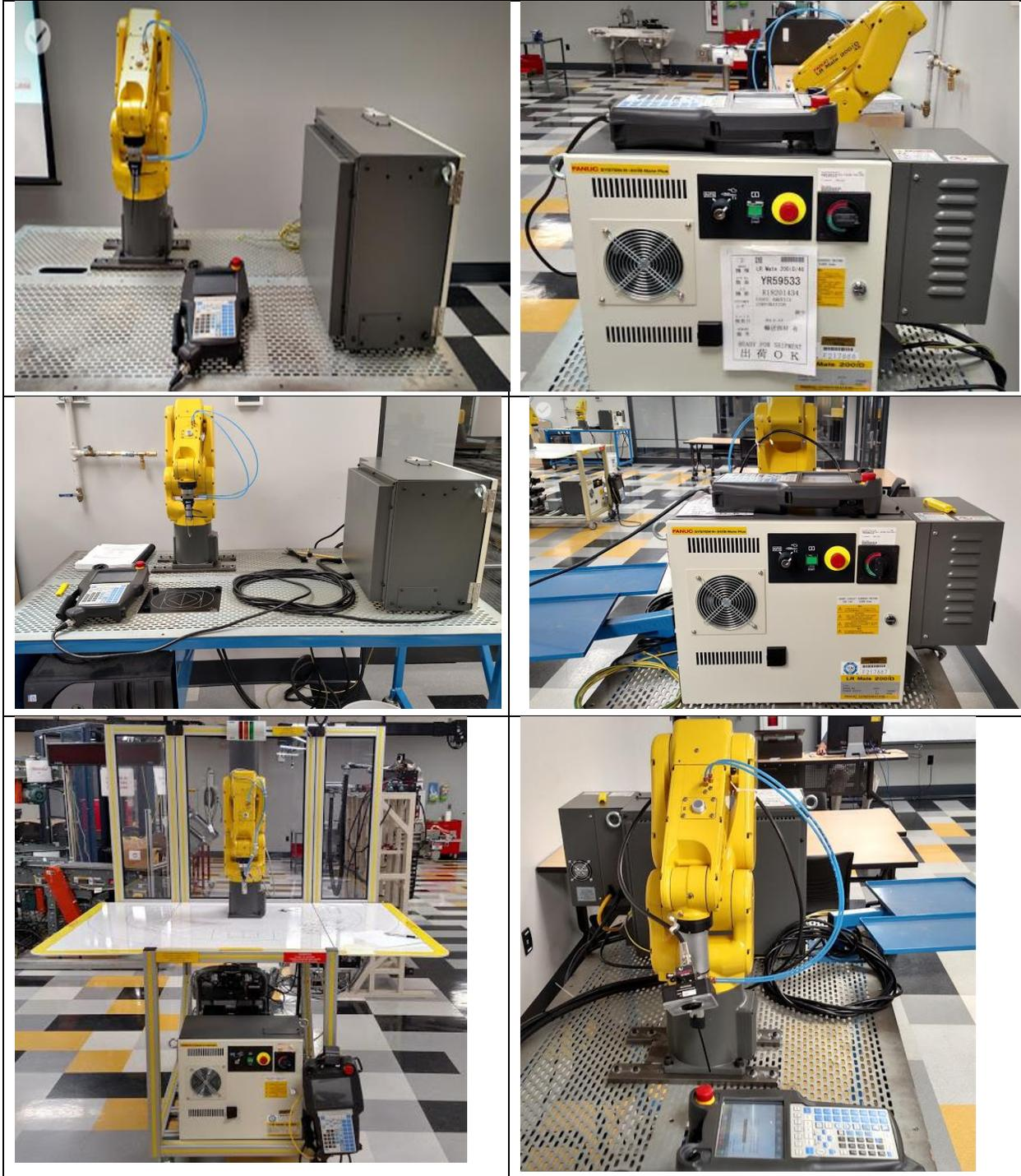
The LR Mate 200iD/4s is a compact robot with the approximate size and reach of a human arm (550mm). The design of the arm minimizes interference to peripheral devices and allows operation in suitable spaces. The advantages of having this type of robot are as follows. Lightest mechanical unit in its class and enables easy system integration and installation flexibility with multiple mounting methods [4].
