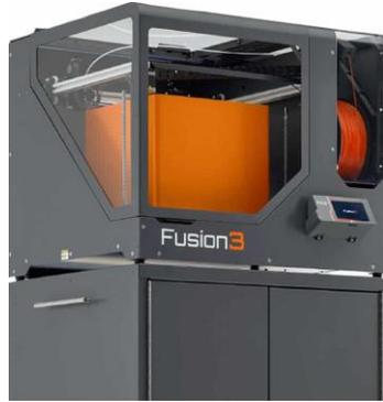
Figure 5: Fusion 3D printer used to print the 3D Blade. Courtesy fusion 3D printer <sup>10</sup>.
