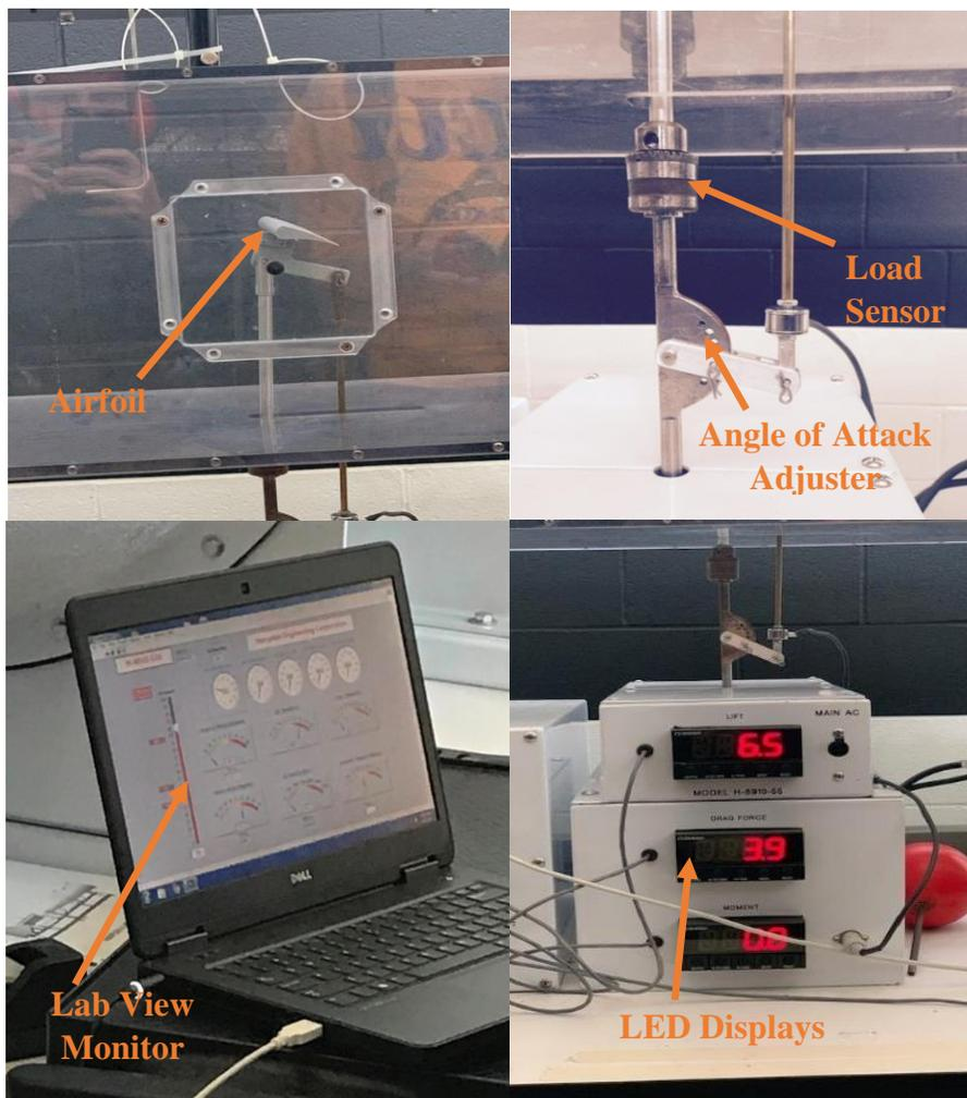
Figure 8: Locking, Pitch Angle adjuster, and load Sensor
