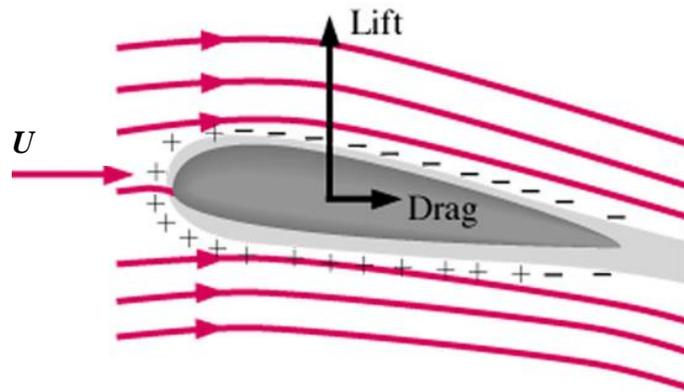
Figure 1: Airfoil cross-section with aerodynamics forces. Courtesy Cengel [9]
