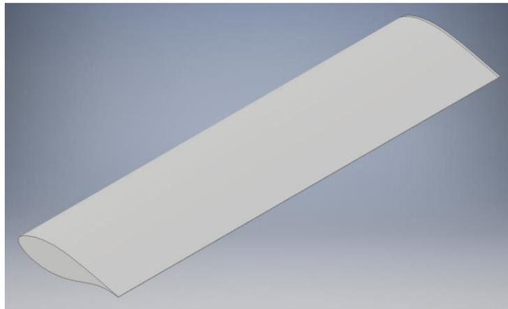
Figure 3: 3D Model of Blade extruded from DU airfoil
