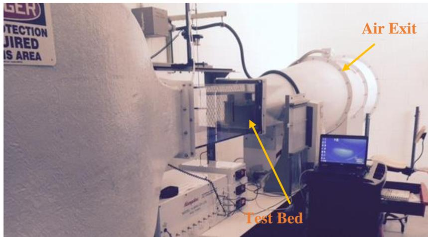
Figure 7 :Wind Tunnel air exit and test bed
