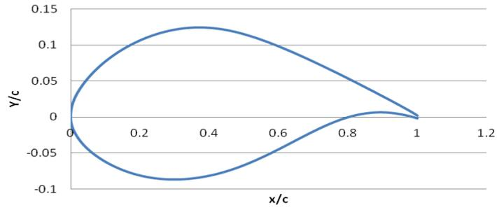
Figure 2: DU airfoil and blade cross-section
