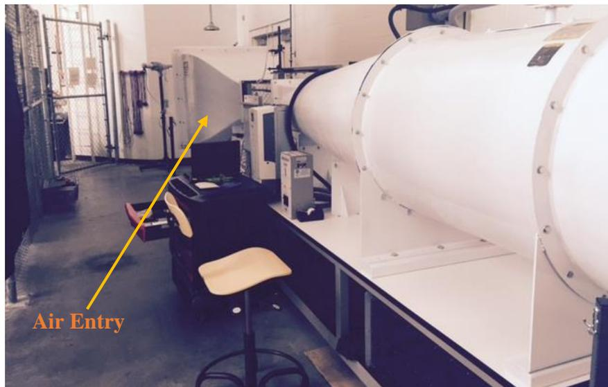
Figure 6: Wind Tunnel showing air entry
