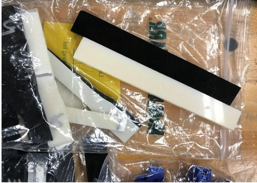
Figure 2: CNC machined cut-to-size specimens for hardness test
