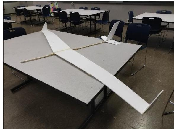
Figure 5. Completed glider from the modified course section (7 ft wingspan)
