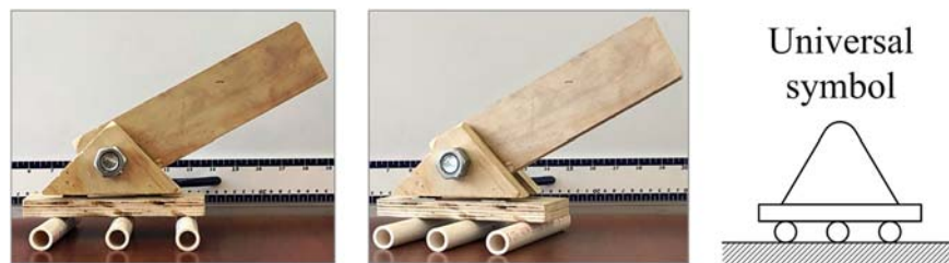
Figure 5. Roller support and universal symbol
