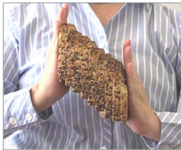
(a) Shearing of bread beam (b) Positive shear representation
