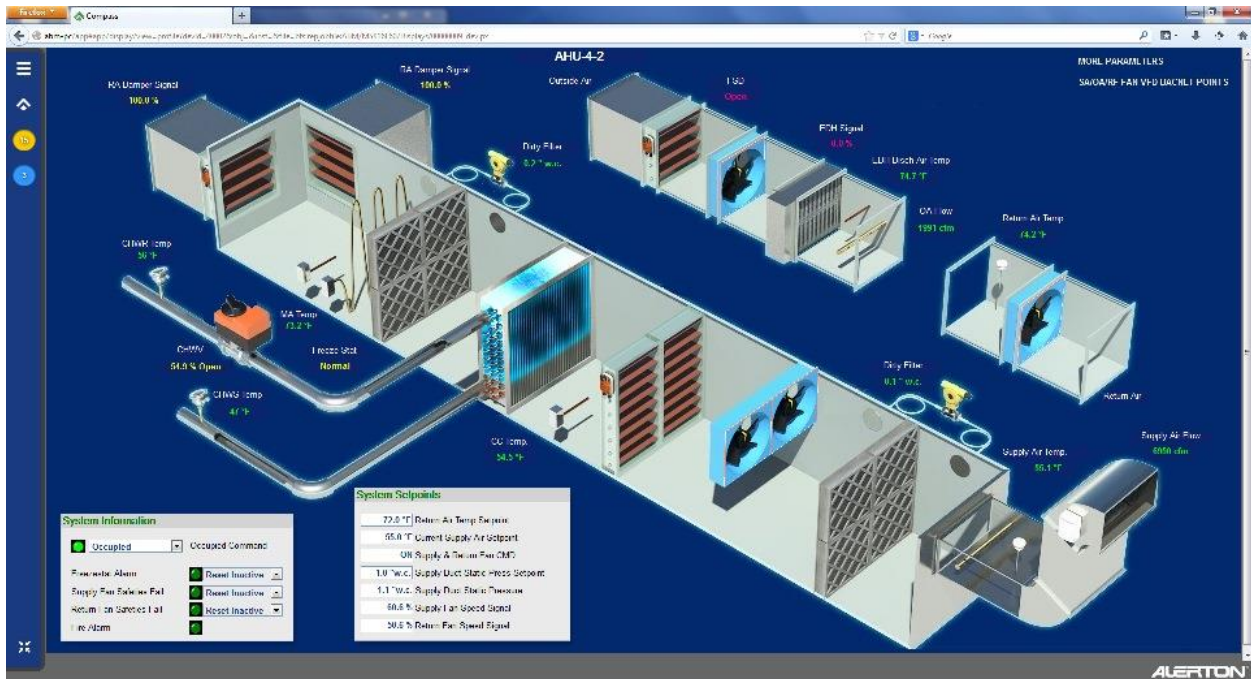
Figure 8: The BAS interface, showing an AHU of a specific building
