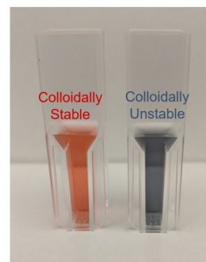
Figure 2: Gold nanoparticle solutions which are colloidally stable (left) and aggregated (right).
