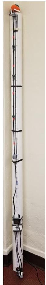
Figure 2: Falling Ball lab set-up
