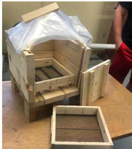
Figure 4. Completed Phase 2 solar-powered food dehydrator design #1; food trays are stackable.
