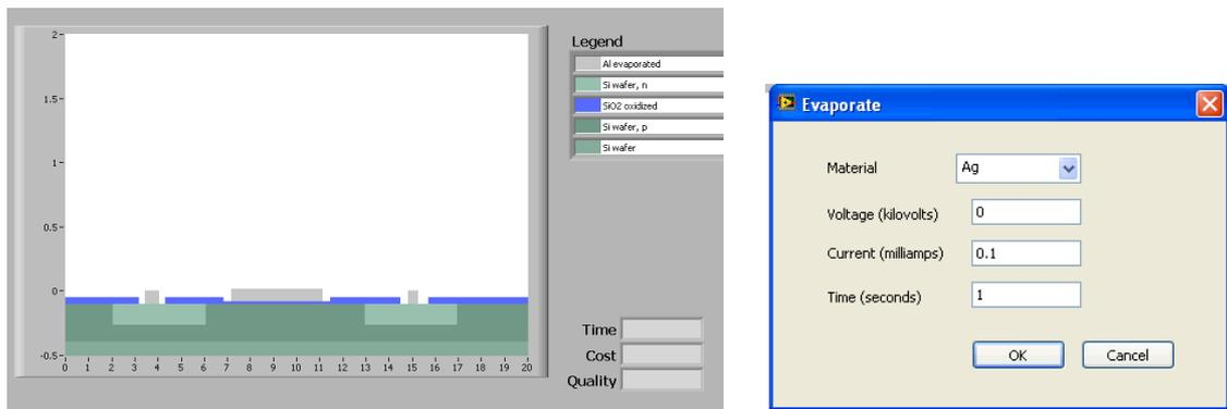
Figure 3: Virtual Nanofab trainer's main screen showing a MOS transistor fabrication process.
