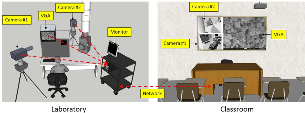
Figure 1: This is the concept diagram as proposed in the NSF-NUE proposal, linking the laboratory to the classroom.
