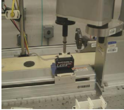
Figure 6: Conveyor-belt inspection of solar cells using CCD camera and laser light scattering.
