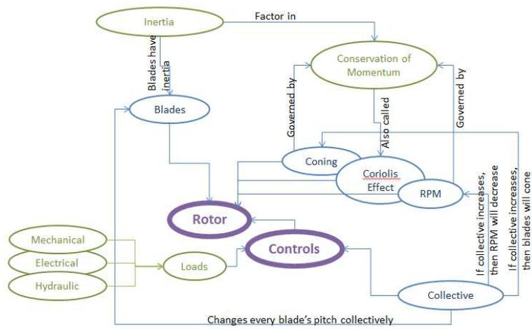
Figure 4. Detailed concept map of rotor with Good-to-be-Familiar-With Conservation of Angular Momentum and Control Loads.
