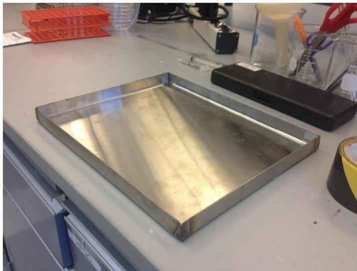
Figure 3. The casting tray made specifically for the Creation of Dissolvable Strips Lab.
