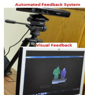
Figure 5: Example setup of AFS with visual feedback for students
