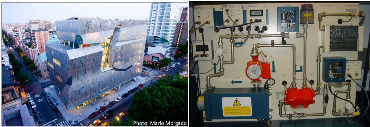
Figure 1. (a) 41 Cooper Square. A new LEED Platinum certified academic building is used as a context to explore control system concepts. (b) Temperature Process Control Rig. Students apply feedback control principles to control the primary and secondary flow rates through a heat exchanger.
