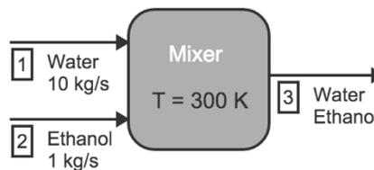
The streams and process units are then connected, and the process flow diagram is complete.
