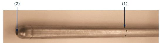
**Figure 1 :** Image of a pitot tube showing the ports along the side (1) measuring the pressure of the moving fluid and the port at the end (2) measuring the stagnation pressure.
