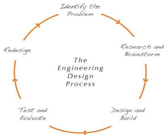
Figure 2. The Engineering Design Process used in the Curriculum ([www.waterbotics.org](http://www.waterbotics.org))
