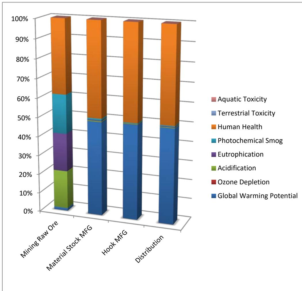
Figure 1 – Total Life Cycle Impacts (Courtesy Joshua Kingston, Life Cycle Assessment of High Carbon Steel Fishing Hooks Manufactured for Saltwater Fishing, Term Paper, Texas University, August 2016)
