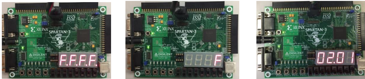
Fig. 3 (a) Without time-multiplexing module, all 4 LED displays always show the same digit (e.g., F); (b) With time-multiplexing module, the rightmost LED display is enabled only to show F; (c) With time-multiplexing module, 4 LED displays show a different digit on each.
