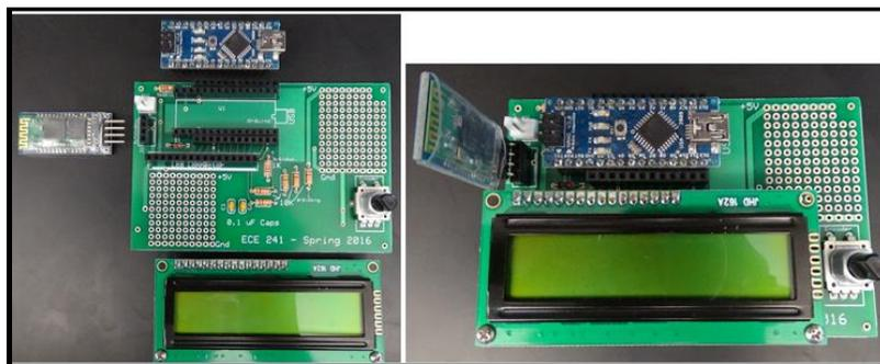
Figure 4. Prototyping board designed in house.
