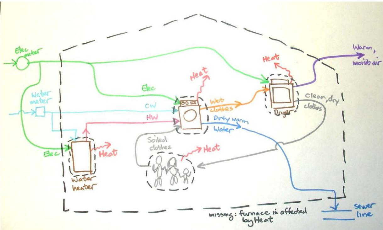
Figure 7 System schematic of a clothes washing system
