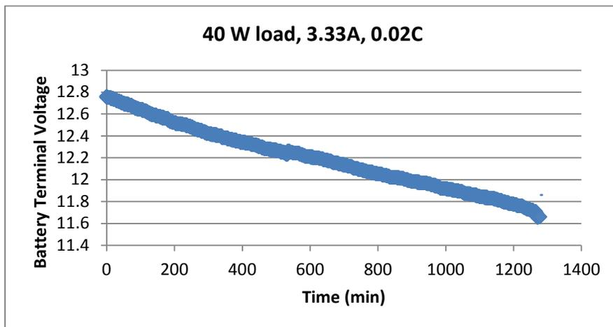
Fig. 16: Battery Discharge Curve (0.02C)
