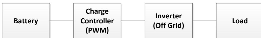
Fig. 13: Off-Grid Setup
