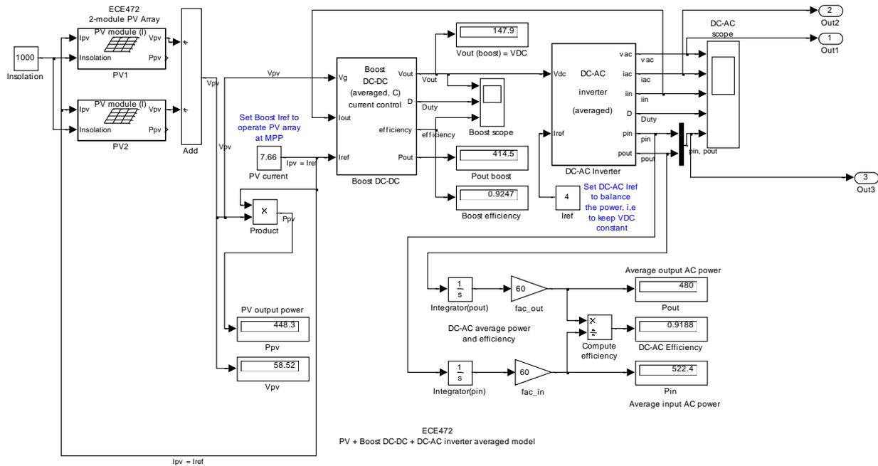
Fig. 3: Simulation Setup
