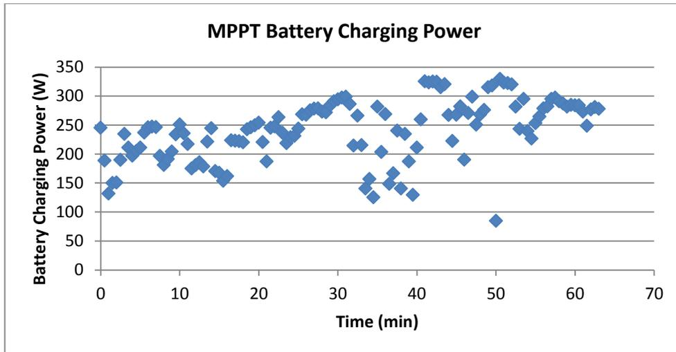
Fig. 18: MPPT Battery Charging Power
