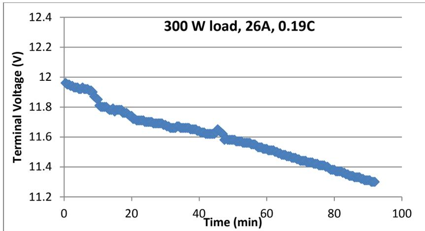
Fig. 15: Battery Discharge Curve (0.19C)
