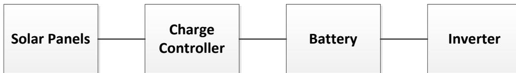
Fig. 10: Charge Controller System Integration Configuration
