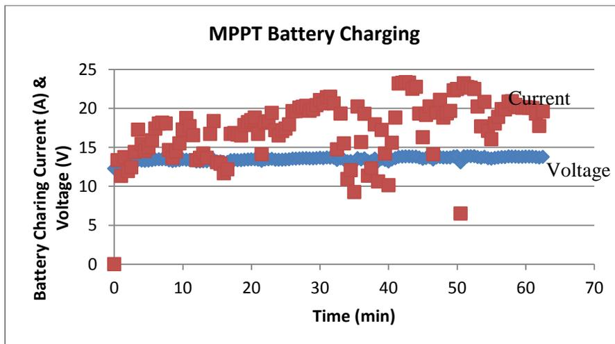
Fig. 17: MPPT Battery Charging Voltage and Current
