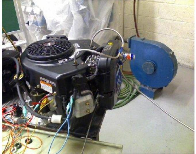
(b) Engine Showing Solenoid Valve
