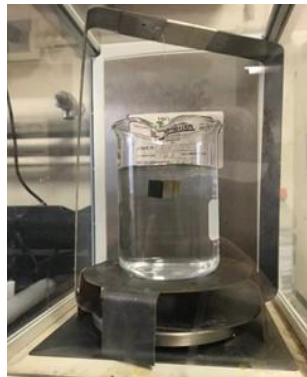
Figure 7: Testing Apparatus inside Analytical Balance used for Density Determination
