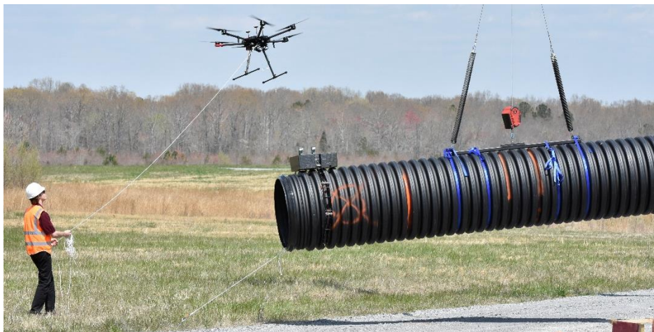
Figure 2: Picture of device grappling a statically hanging large debris (21' X 3') upon contact
